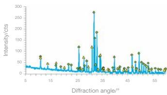
Safety by phase purity – x-ray spectroscopy of maxresorb®, Prof. Dr. C. Vogt, University of Hanover, all peaks can be assigned to HA (yellow) or  $\beta\text{-TCP}$  (green).
